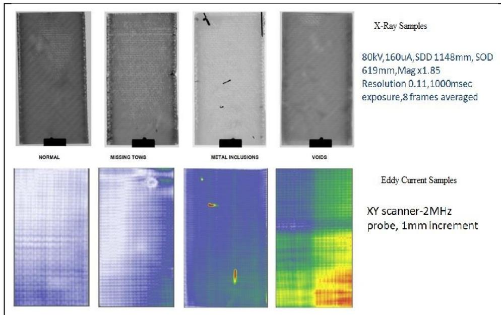
**Figure 4** X-Ray and Eddy current scans of 4 flawed 3D woven samples
