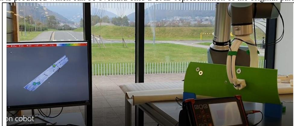
**Figure 9** robot setup with curved 3d printed sample and robot programming software
