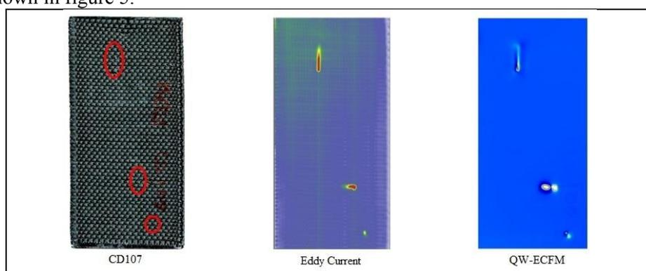
**Figure 5** A 3D woven sample analysed by both eddy current and QW-ECFM
