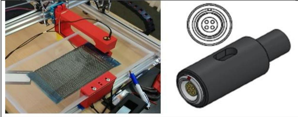
**Figure 2** Ether NDE eddy current scanning equipment
