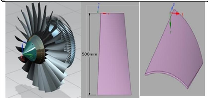
**Figure 11** CFM56 engine compressor blade schematics
