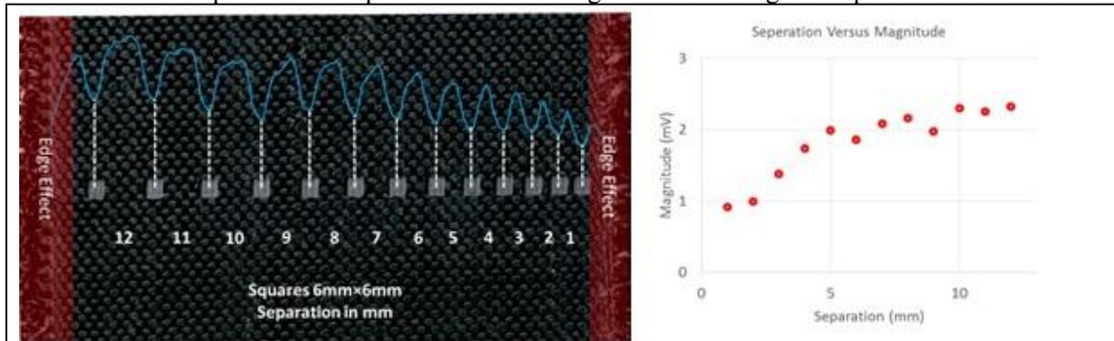
**Figure 8** Reference Sample 2 scanned with QW-ECFM
