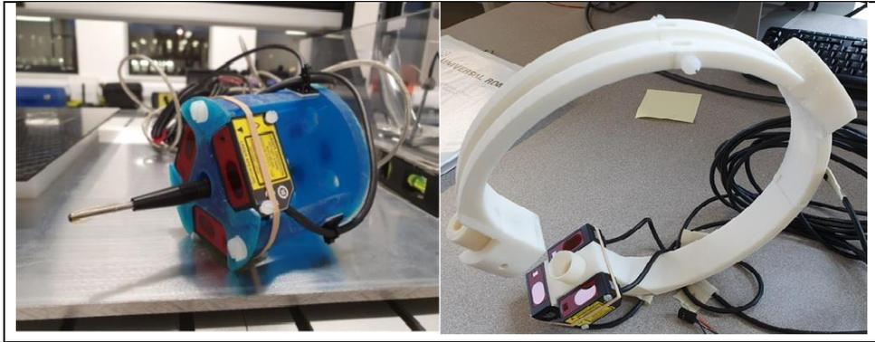
**Figure 10** Eddy current sensors holder designed by TWI
