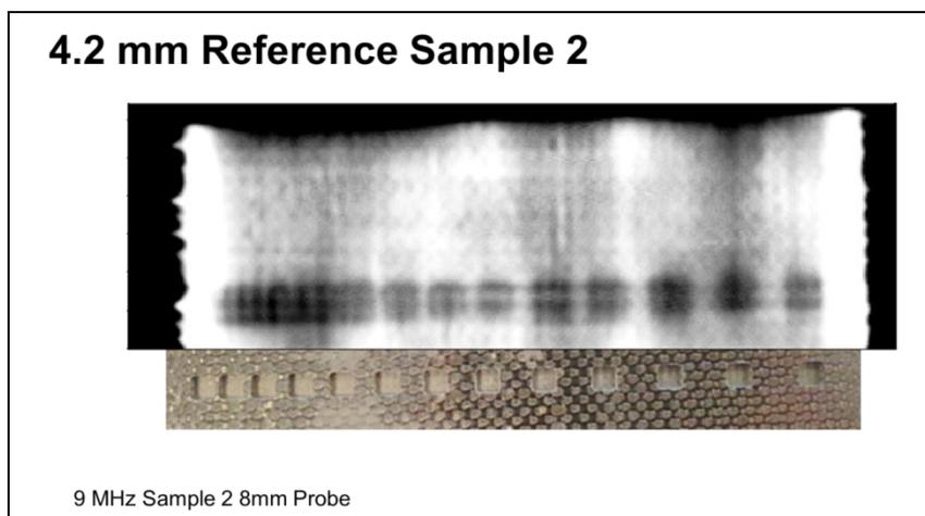
**Figure 7** Reference Sample 2 scanned with eddy current
