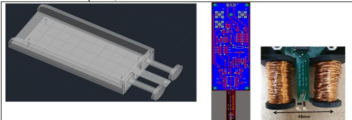
**Figure 3** AHS Quantum Well Hall Effect Eddy Current Field Measurement (QW-ECFM) scanning head
