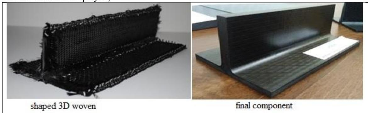
**Figure 1** typical 3D woven shaped fabric/composite
