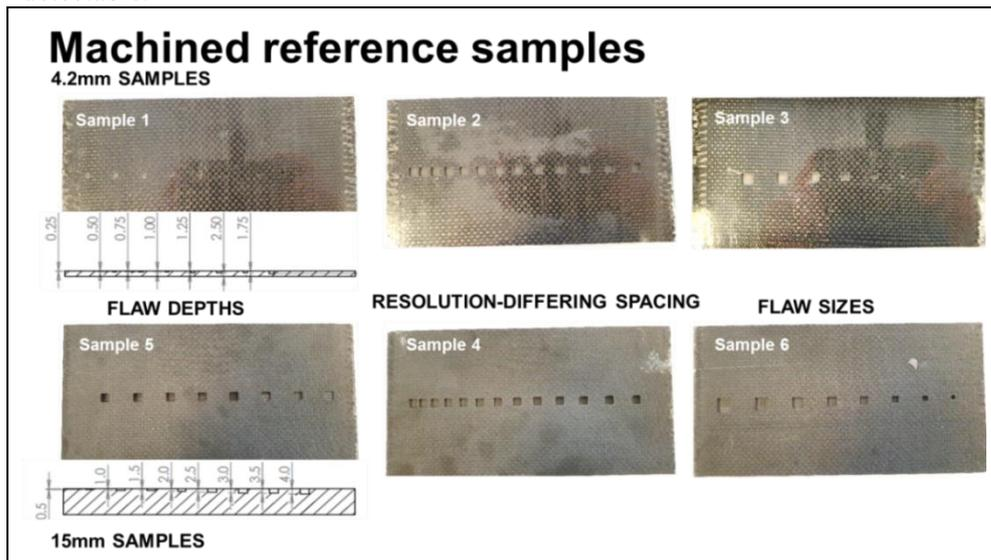
**Figure 6** The reference samples made for this project
